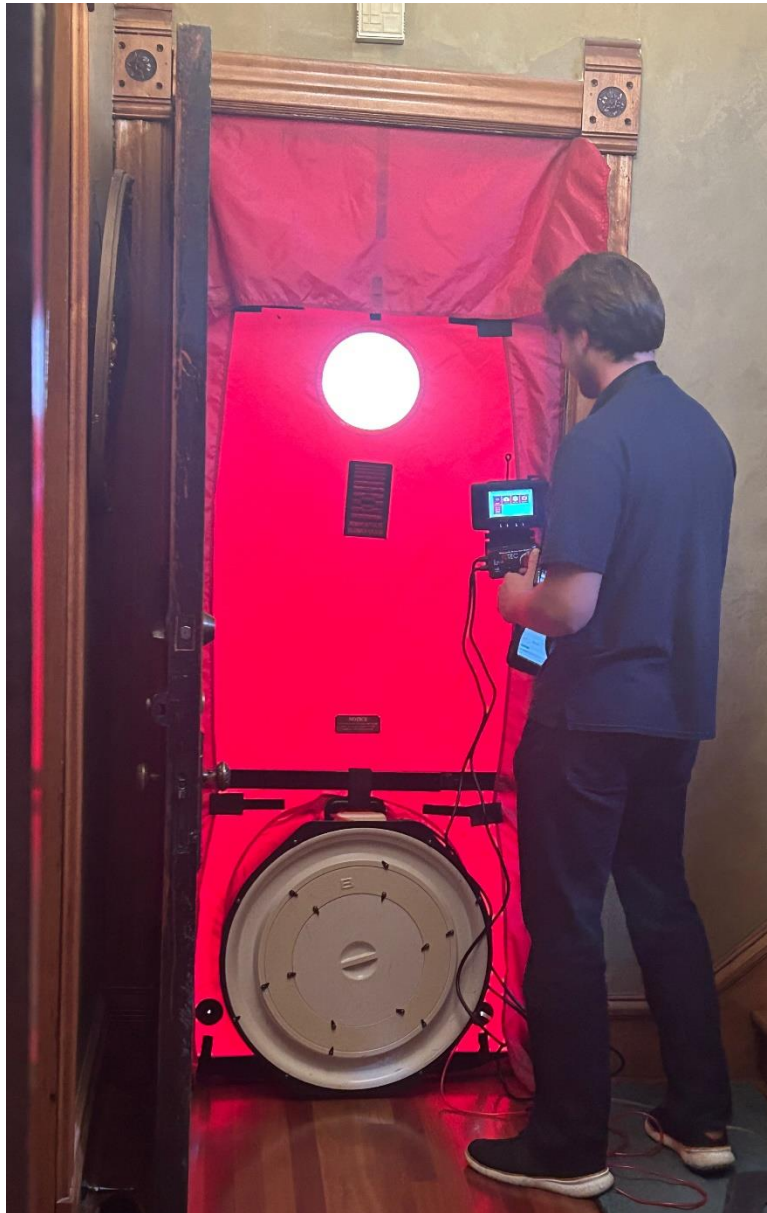
Figure 7. Example of a blower door test.
