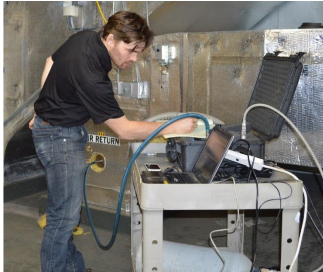
Figure 14: A CO 2 -based tracer gas system was used to measure flow rates and air leakage between air streams where necessary
