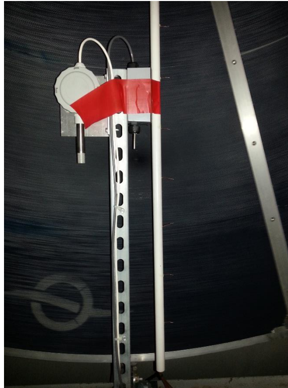
Figure 12: Measuring radial variations in outlet temperature distribution with respect to controlling sensors
